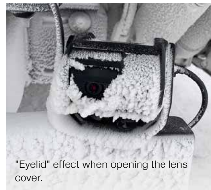
Camera ready for use even during snowfall due to shutter housing.
